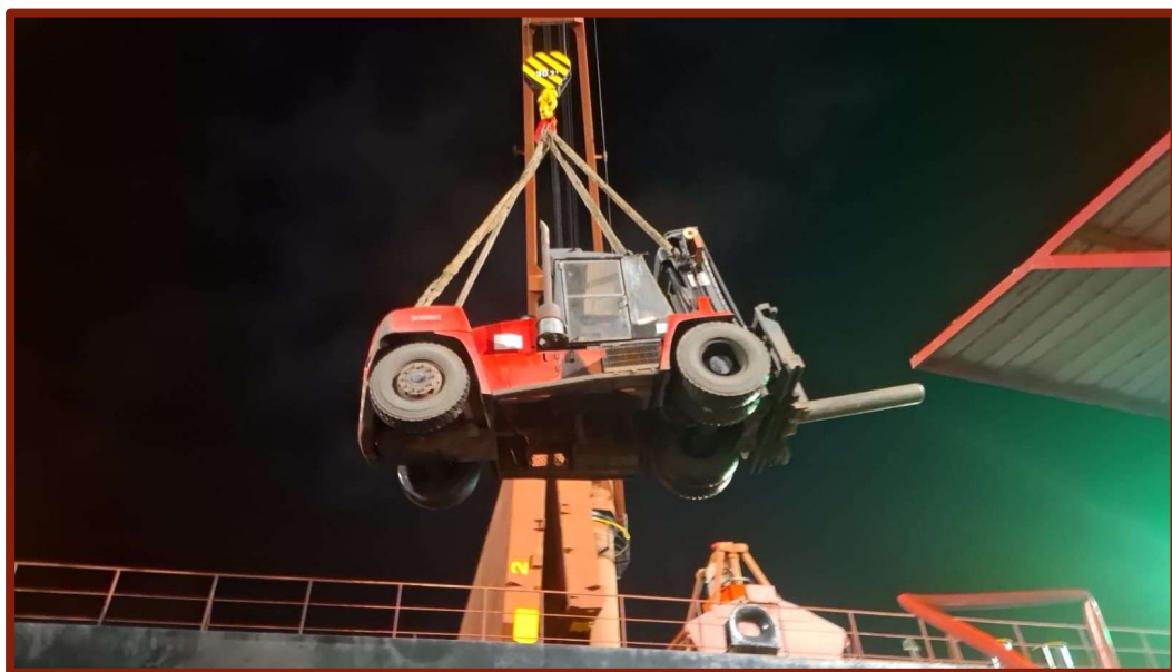
Shore forklift being lifted onto holds to handle light and heavy coils in Sao Francisco do Sul, Brazil.
