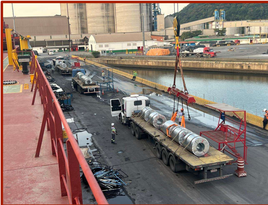
Manual spread-bar discharging steel coils onto trucks alongside. Sao Francisco do Sul Port, Brazil.
