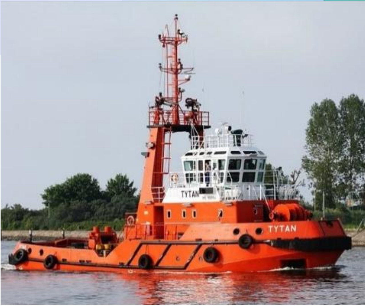
TUGBOAT TYTAN (FF 1) 600 m 3 /h barrier Expandi 300 m 4 firefighters
