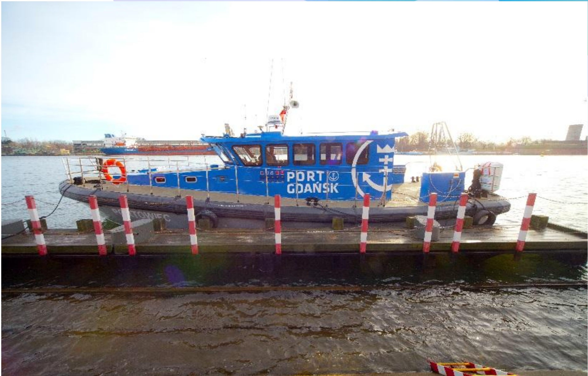
"PORTOWIEC" Length: 14,95 m Width: 4,7 m Draft: 1,5 m Freeboard: 2,09 m
